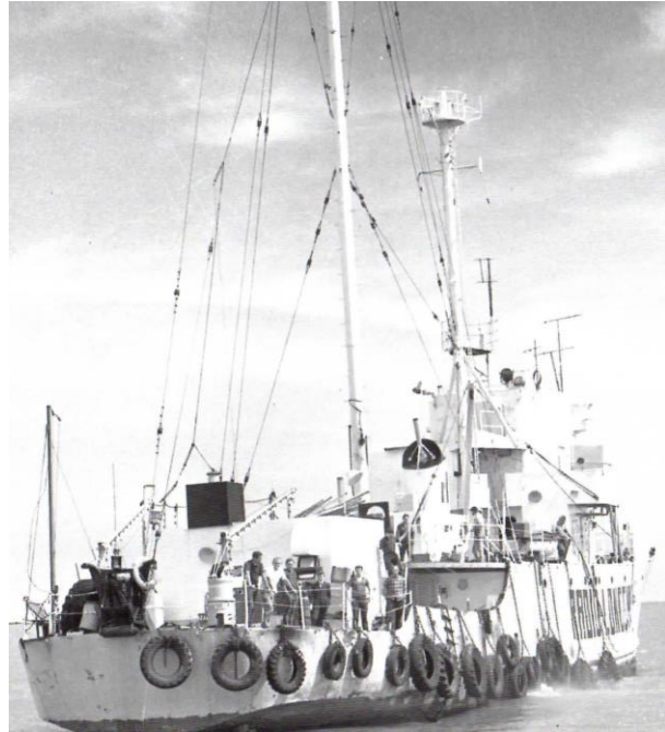
Figure 4. The Radio London ship MV Galaxy in 1966. The ATU box and output termination are visible on the roof of the transmitter room
